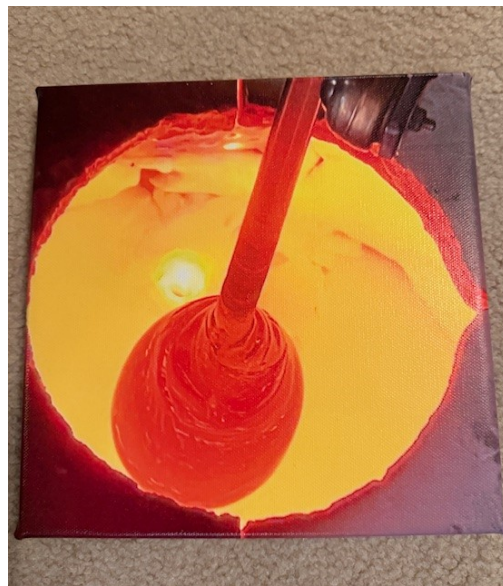
Above, molten glass ready to be blown into a vase
